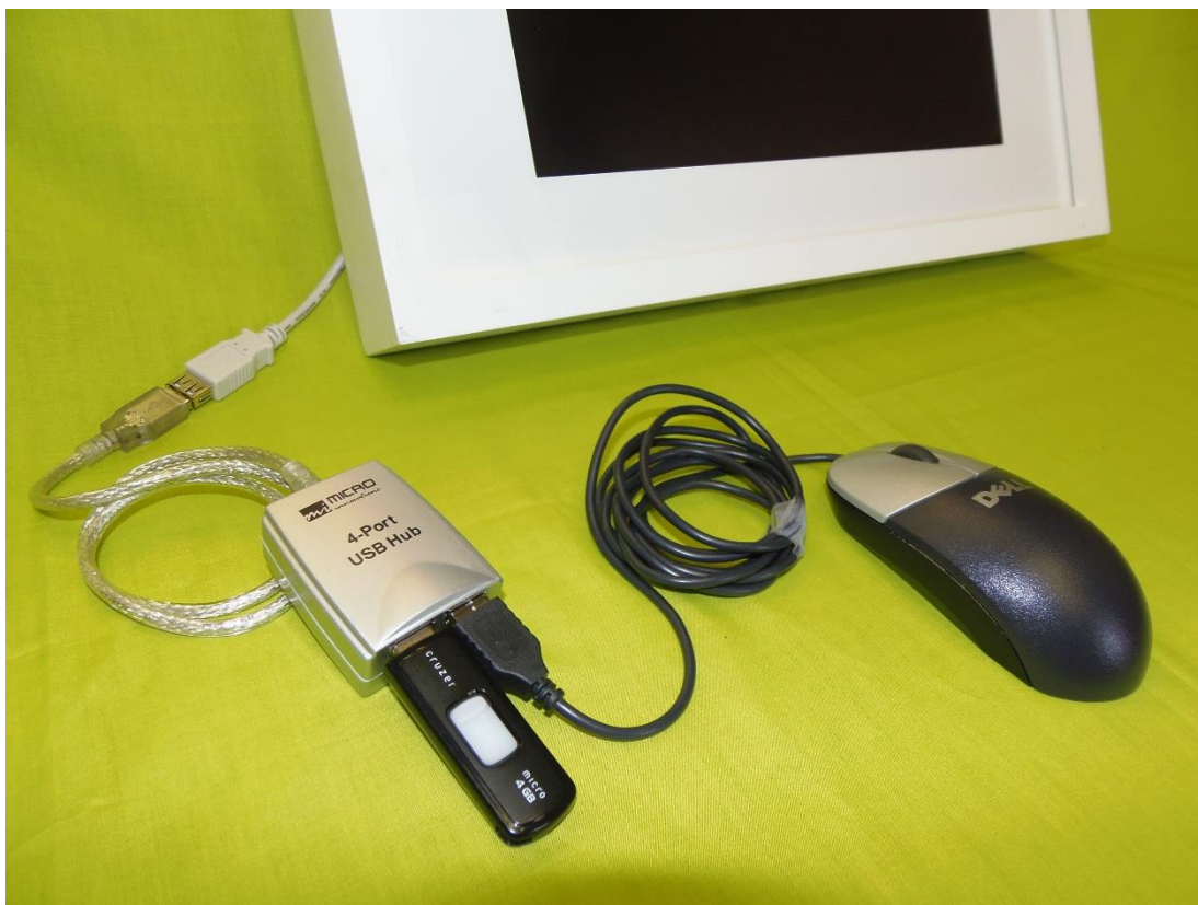
Figure 10. A mouse and USB flash drive connected to the digital platform via a USB hub.
